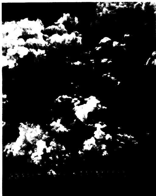
Fig. 5. SEM of powder deposited on the reaction vessel walls upon photolysis of [(C_2H_4)_2RhCl]_2 for 8 h.
